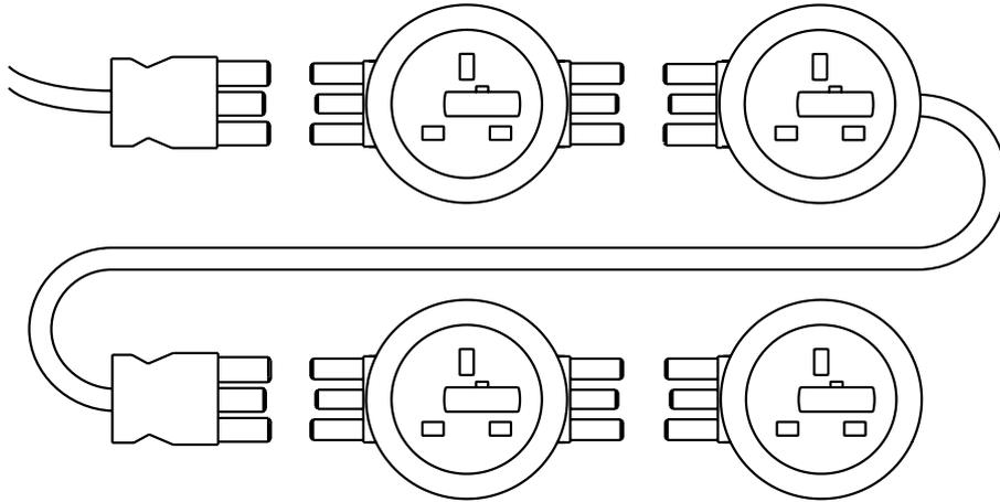
Connectors can rotate through 90°, offering easy installation and low profile wiring for a wide array of applications.
