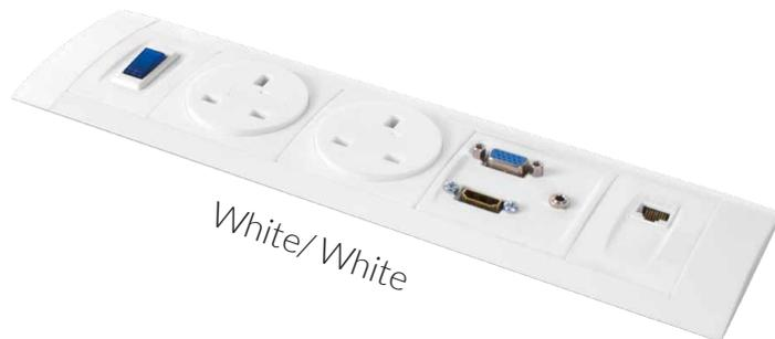
An extraordinarily low profile power & comms unit which fits flush to a table top. As well as the power, data & AV options being customisable, sockets can be orientated to service users on both sides of a table. Thin profile makes it suitable for panel mounting and soft furnishing.
