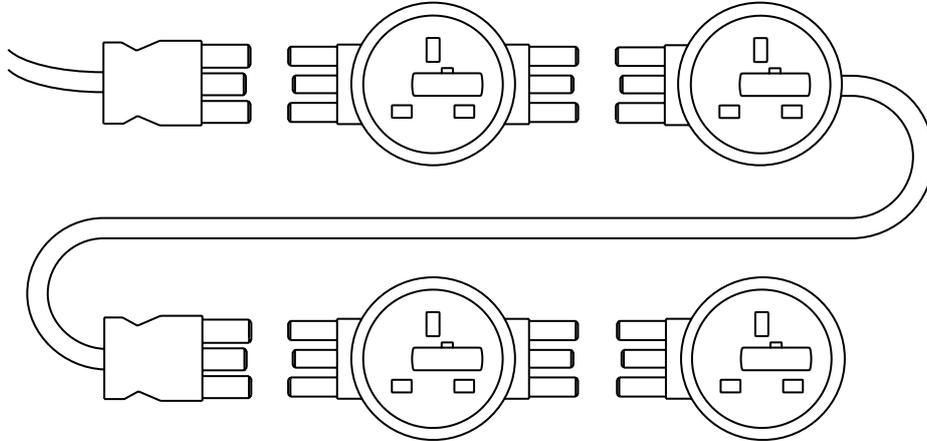
Connectors can rotate through 90°, offering easy installation and low profile wiring for a wide array of applications.
